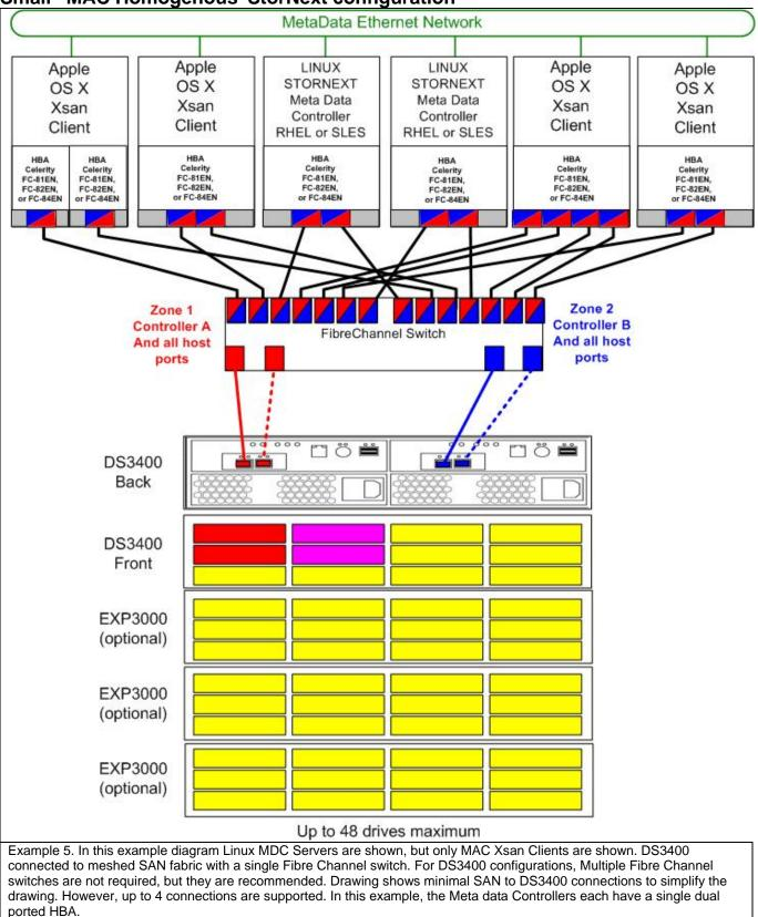
RAID 1 pairs for Meta Data and Journal are represented. Global Hot spares would be assigned as appropriate. While SAS drives would be recommended for Meta Data and Journal, SAS and/or SATA drives could be used for data as appropriate.
